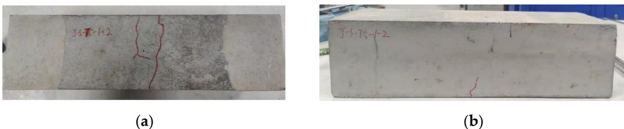
**Figure 6.** Typical fatigue failure of reinforced concrete specimens (RC series): (a) bottom surface; (b) side surface.
