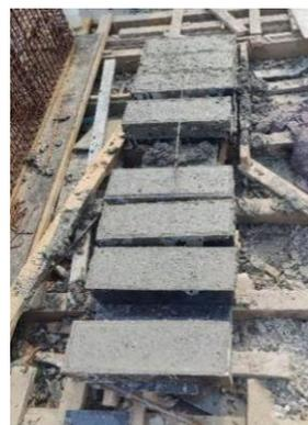
**Figure 2.** Specimen preparation during concrete pouring.
