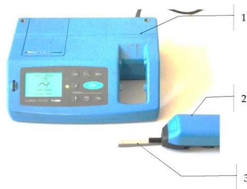
**Figure 4.** Surface roughness measurement by the Hommel tester T1000: 1—signal analysis device; 2—measuring head with needle; and 3—measured sample.
