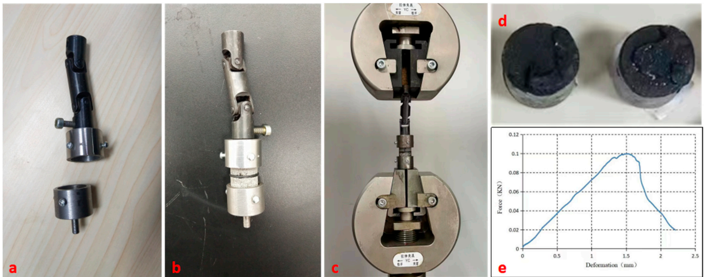
Figure 3. Testing of asphalt mastic–aggregate interface specimens: (a) holding fixture; (b) specimen fixed by holding fixture; (c) specimen fixed into universal testing machine; (d) specimen failure surface; (e) loading curve.
