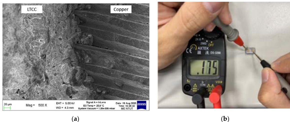
Figure 12. SEM image of the microstructure of the interface between the LTCC ceramic and copper (a) and the electrical conductivity test (b).
