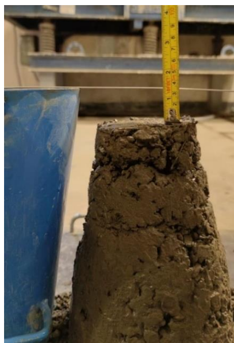
Figure 1. Slump test of the M_3 concrete mix.
