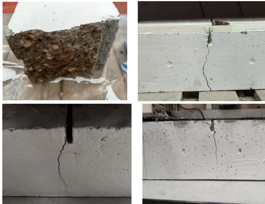
Figure 7. The post-crack of the concrete specimen after the bending test by contrast (left upper is M0, right upper is M1, left bottom is M2 and right bottom is M3).
