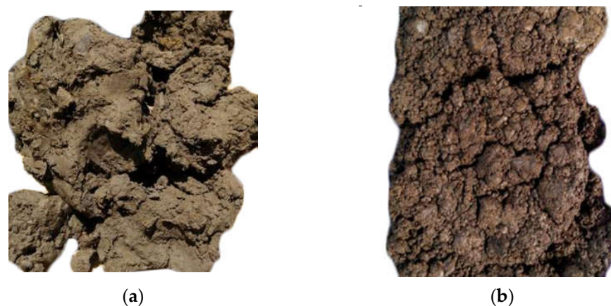
Figure 3. Photograph of soil sample. (a) clayey soil sample; (b) weathered basalt soil sample.
