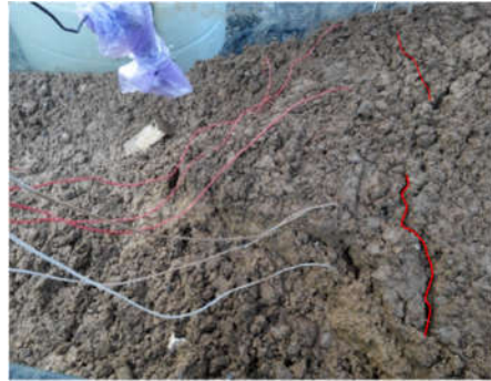
Figure 7. Tension cracks on the slope surface (Test 1).
