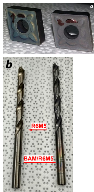
Figure 1. Photos of the commercial industrial tools used for the experiments. (a) Two WC-Co-based cemented carbide turning inserts processed with a BAM coating. Right is the BALINIT LATUMA TM (AlTiN) specimen. (b) Untarnished and BAM-coated R6M5 drill bits.
