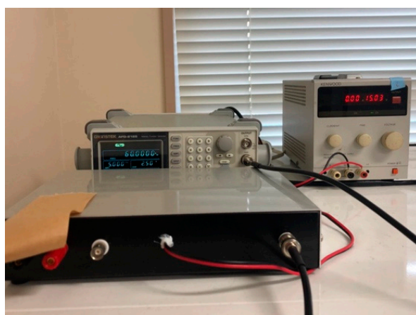
Figure 2. The control system of experimental apparatus.
