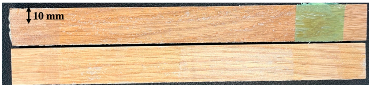
Figure 16. DCB specimens' fracture surfaces.
