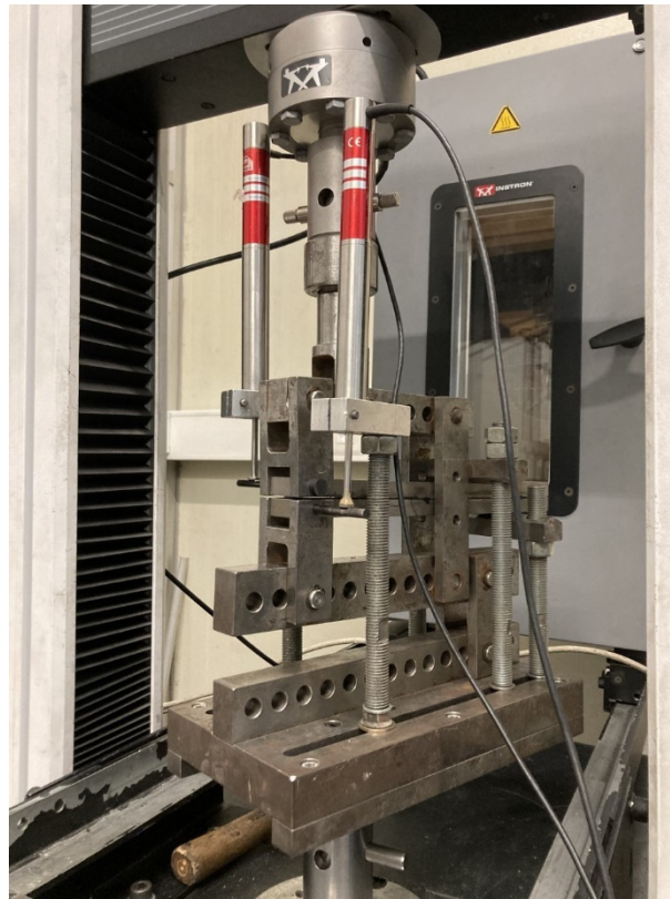
Figure 7. Apparatus for mixed-mode test.
