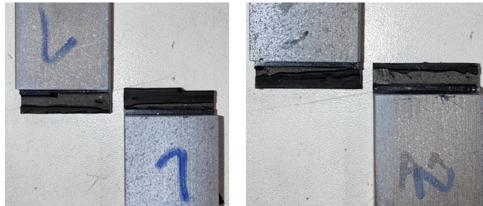
Figure 12. Failure mode for two TAST specimens.
