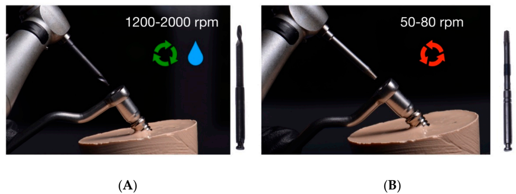
Figure 4. Mechanical technique of fractured abutment screw removal using the Sanhigia ® extractor kit. (A) First drill and guide fixed on the dental implant connection. (B) Second drill.
