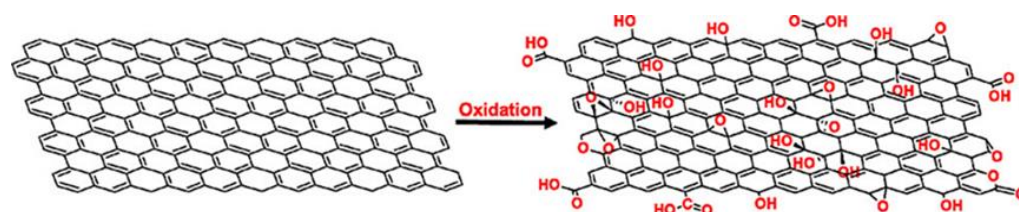
Figure 1. Oxidation of graphene to form graphene oxide. Reprinted from [19].
