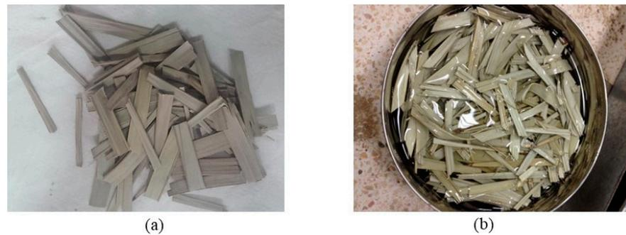
**Figure 2.** Local date palm leaves fibers used in the study: (a) dry; (b) soaked.
