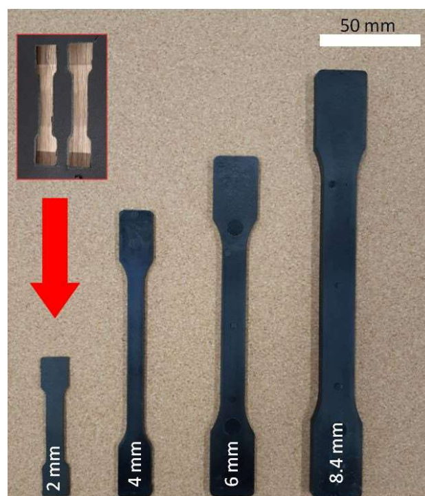
Figure 2. Tensile testing samples at four different thicknesses: 2 mm; 4 mm; 6 mm, and 8.4 mm (from left to right). 2 mm thick samples were cut from the industrial element (red frame and arrow) while 4 mm; 6 mm and 8 mm thick were directly injection molded.
