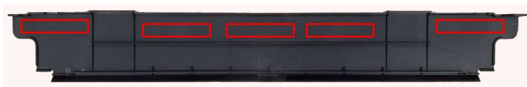
Figure 1. Industrial automotive element with marked places (red frames) from which 2 mm thick samples were cut and analyzed.
