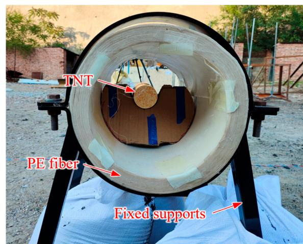
Figure 1. Photograph of the previous experimental setup.
