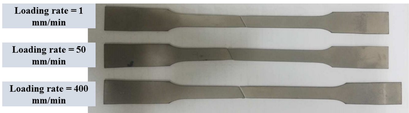
Figure 4. Fractured dumbbell-shaped samples under different loading rates.
