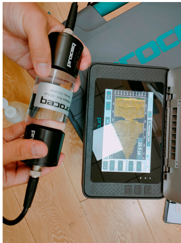
Figure 9. Ultrasonic non-destructive testing equipment.
