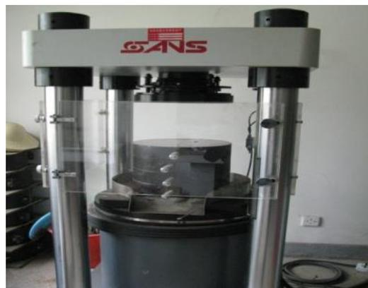
**Figure 2.** MTS electro-hydraulic servo press.
