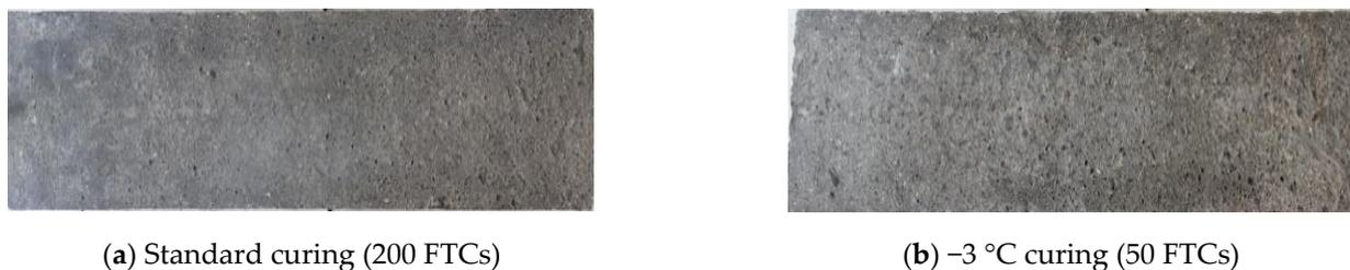
**Figure 5.** Appearance damage of A-2 specimen after FTC under different curing conditions.
