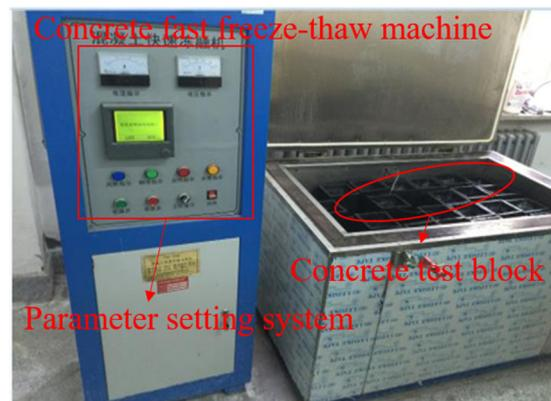
Figure 3. Concrete freeze–thaw circulator.
