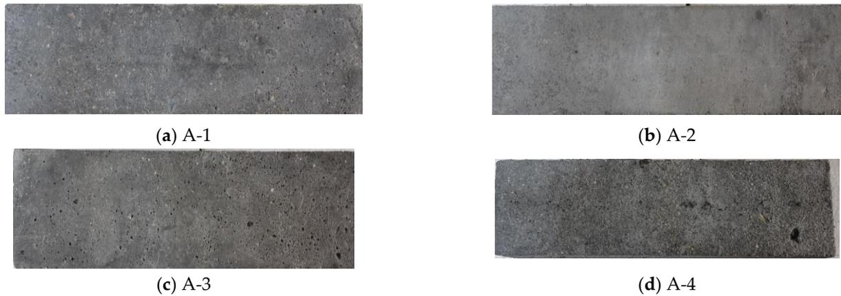
**Figure 6.** Appearance damage of concrete with different gas content after 150 FTCs under standard curing.
