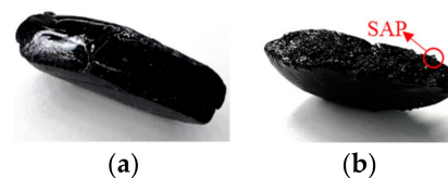
Figure 23. The sections of specimens: (a) the section of the specimen without SAP; (b) the section of the specimen with SAP.
