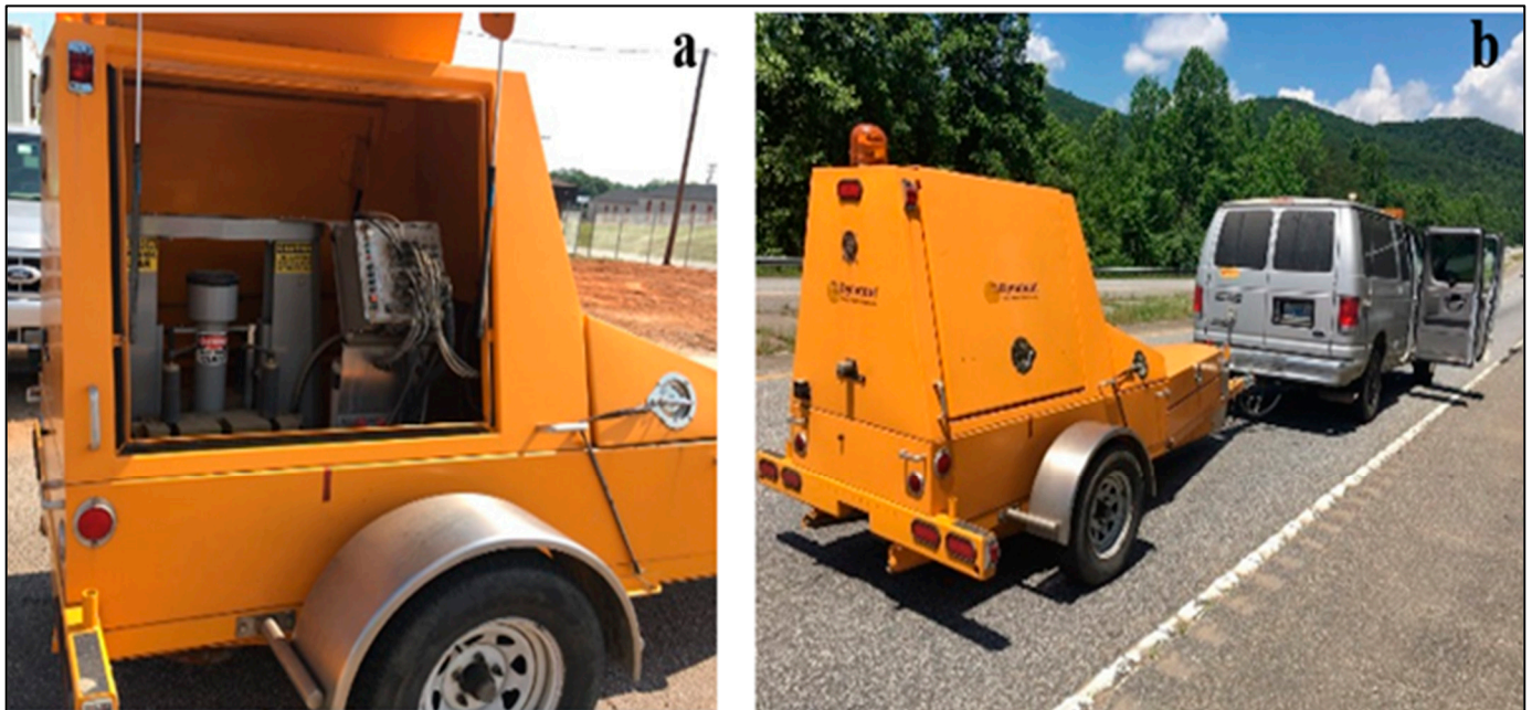
Figure 4. FWD:(a) Loading frame, and (b) system.
