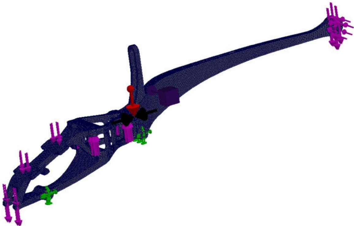
Figure 16. Boundary conditions and loads in frame geometry used in topology analysis, model divided into finite elements.
