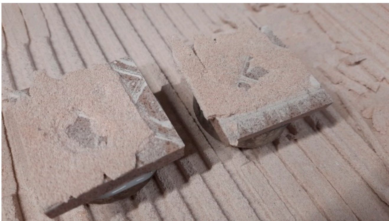
Figure 13. Photo of the samples after tensile-adhesive strength experiment.
