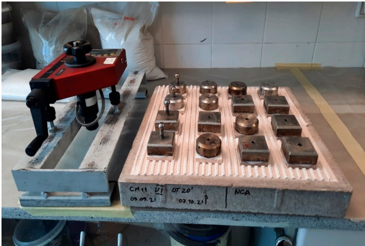
Figure 6. Samples prepared for tensile-adhesive strength experiments.
