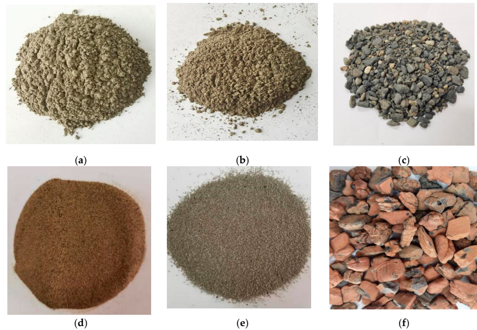
Figure 1. The raw materials: (a) cement; (b) fly ash; (c) RS; (d) DS; (e) FACs; (f) shale ceramsite.
