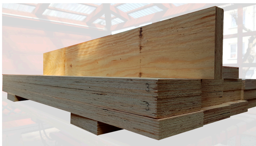
Figure 2. View of the LVL beams.
