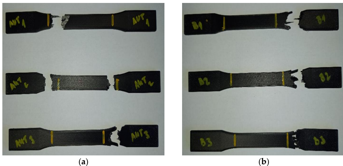
Figure 11. A take on the ruptured samples: (a) type A sample; (b) type B sample.
