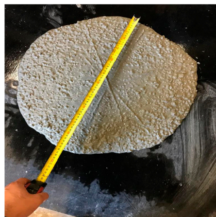
Figure 3. Measuring the slump flow diameter.
