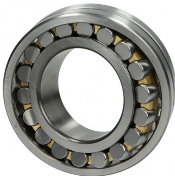
Figure 4. The special series spherical roller bearings (SKF22324VAJ): basic static load—1120 kN; dynamic load—850 kN; and limiting speed—2000 RPM.
