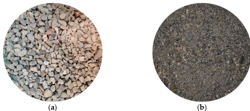
Figure 4. The photo of the aggregate: (a) The recycled coarse aggregate; (b) The fine aggregate.
