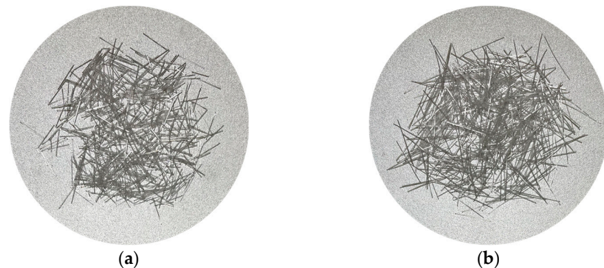
Figure 5. The photo of POM fiber: (a) 6 mm POM fiber; (b) 12 mm POM fiber.
