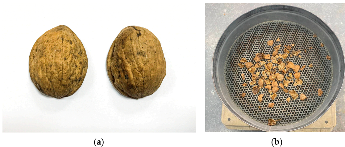
Figure 3. Appearance of the walnut shell: (a) whole; (b) crushed to sizes from 5 to 20 mm.
