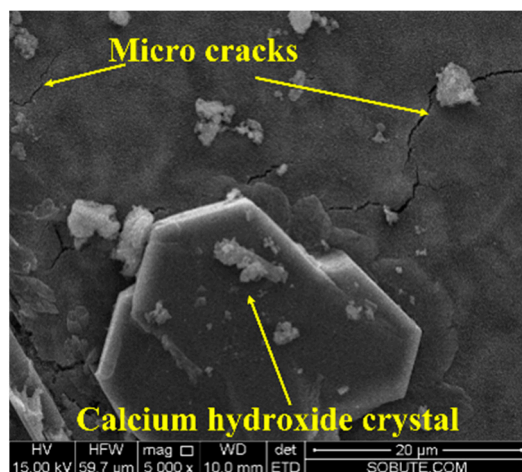
Figure 25. Morphology of cement paste with 6% CaO + 2% 220 s MgO expansive agent ( \times 5000 ).
