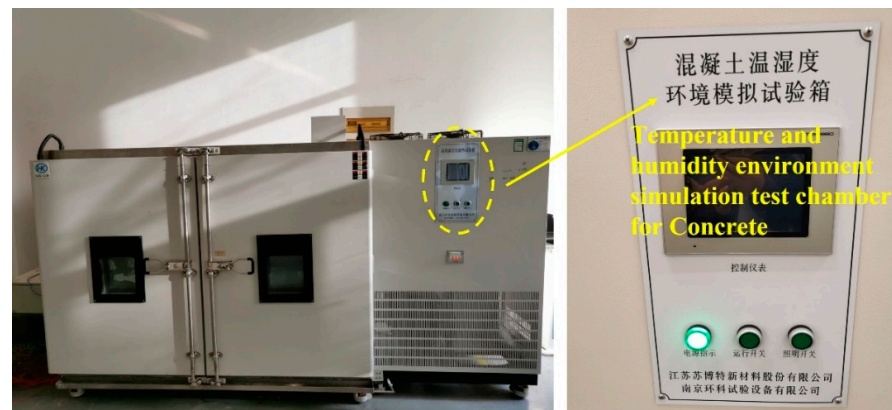
Figure 2. Temperature and humidity environment simulation test chamber for concrete.
