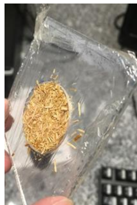
Figure 4. Juncus maritimus fiber placed in spectrometer sample holder apparatus, 30 mm in diameter.
