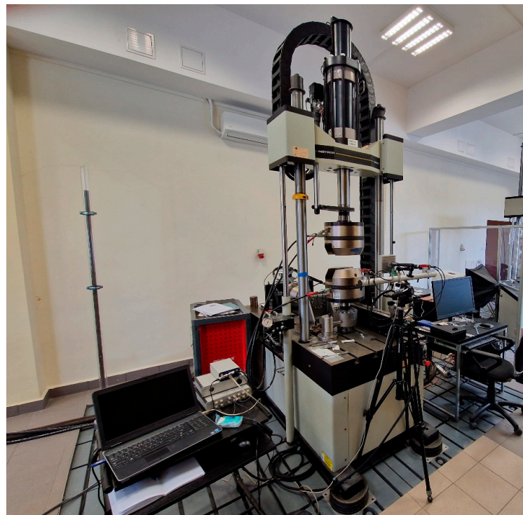
Figure 2. Instron 8802 servo-hydraulic pulsator for three-point bending and compression tests, equipped with the Dantec DIC system.
