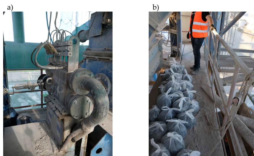
Figure 2. Plant production of asphalt mixtures: Green Pac asphalt foaming system (a), batches of basalt fibers prepared for mixing (b).
