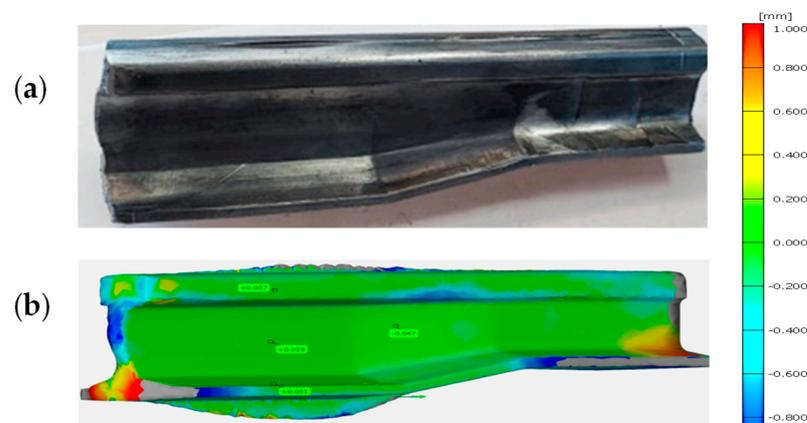
**Figure 11.** Results: (a) a photograph of the lead rail after the last forming operation, (b) a comparison of the shape and dimensions from FEM with the experiment, with a map of deviations (green color is best fit).
