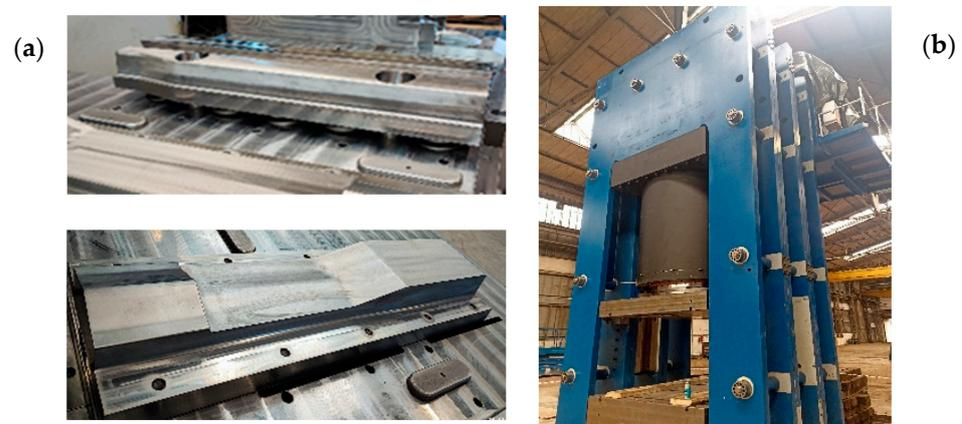
**Figure 20.** Photos of: (a) selected tools used to forge a 60E1A6 profile, (b) the hydraulic press of 5000 tons pressure.
