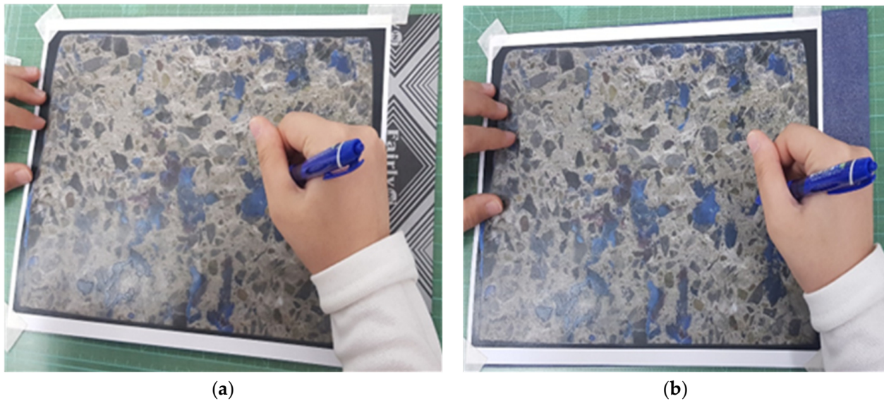
Figure 11. Step 2: modeling the epoxy areas and concrete edges of side (a) A and (b) B.
