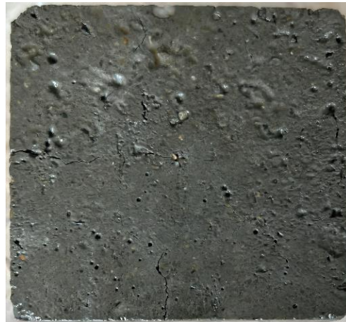
Figure 1. Surface of concrete specimen after pretreatment.
