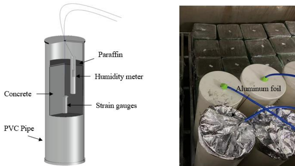
Figure 3. PVC pipe and PVC pipe in a variable temperature curing chamber.
