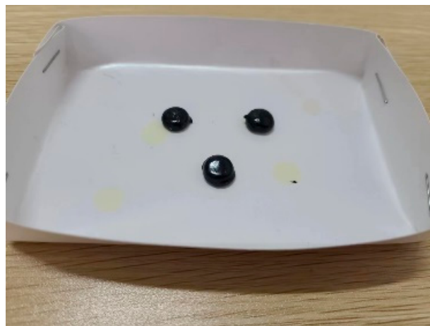
Figure 6. The 8 mm-bitumen specimens used in the LAS and LASH tests.
