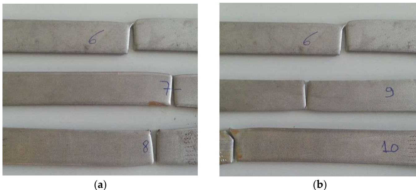
Figure 12. AISI 321 samples at three weeks (a) and three months (b) after the tensile test.
