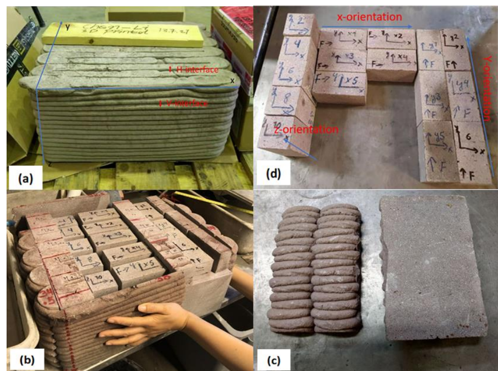
Figure 3. Sampling process (a–d) for printed specimens (5 cm × 5 cm × 10 cm) obtained from the printed concrete slab (38 cm × 36 cm × 22 cm).
