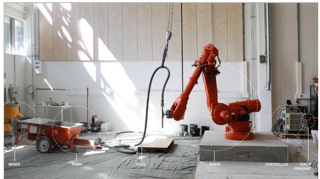
Figure 1. 3D concrete printer.
