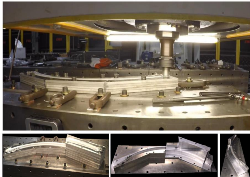
Figure 21. Experimental setup and complex part produced through FSAM by Edison Welding Institute (EWI) (© EWI. reprinted from [125,126] with permission from EWI).
