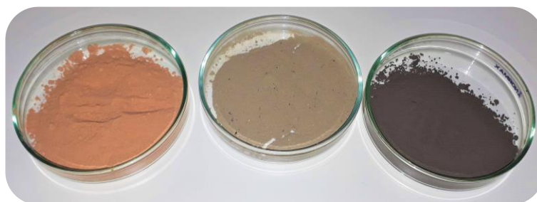
Figure 1. Used GPC precursors. From left to right: MK, BFA, and ground EAFS.
