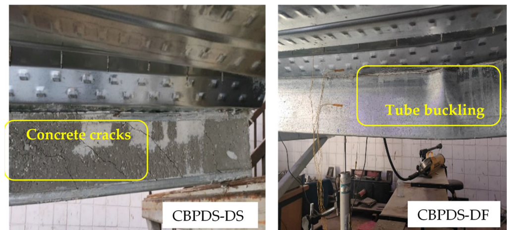
Figure 10. Buckling and concrete cracks for beam in CBPDS specimens.
