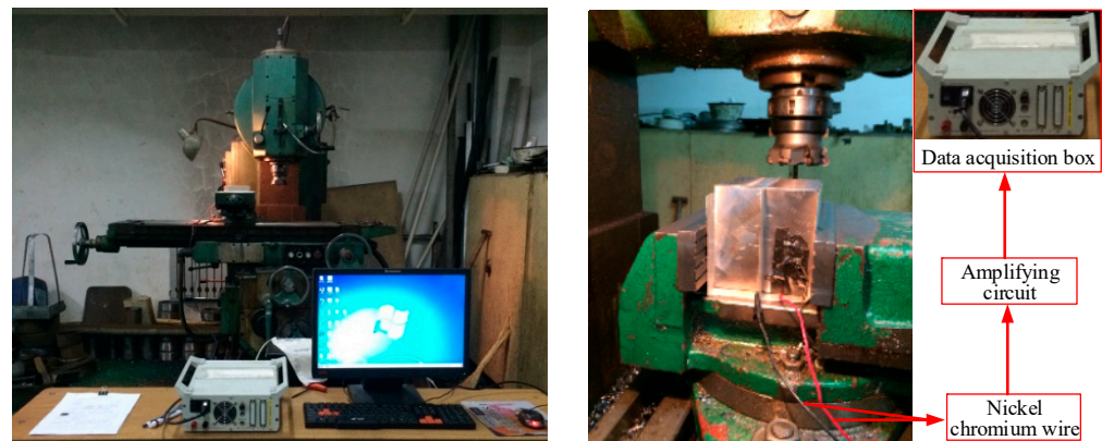
Figure 1. Field diagram of the milling temperature experiment.
