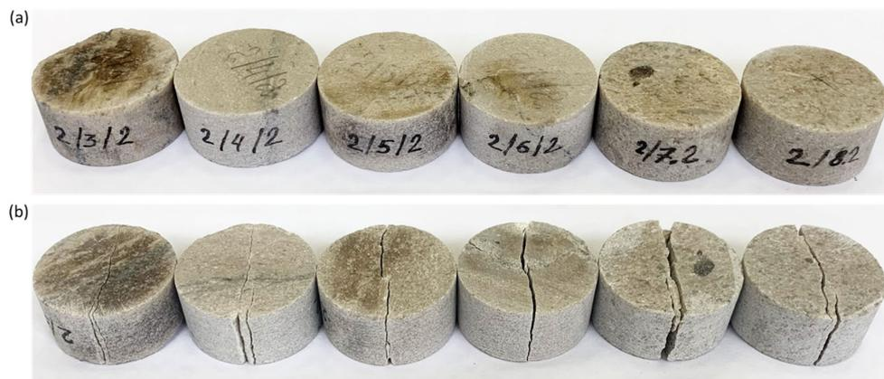
**Figure 11.** Photographs depicting water-wet limestone samples during indirect determination of the tensile strength through the Brazilian test: (a) samples before testing; (b) samples after testing.
