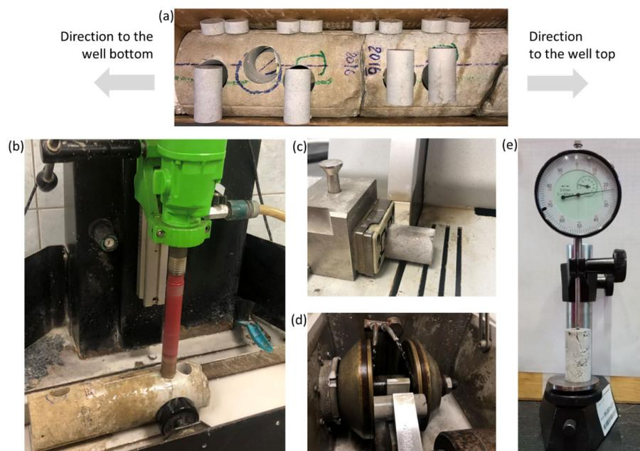
**Figure 1.** Photographs depicting the sample preparation steps: (a) the core from a production well; (b) drilling out the sample; (c) cutting the sample; (d) grinding the ends of the sample; (e) sample measurement.
