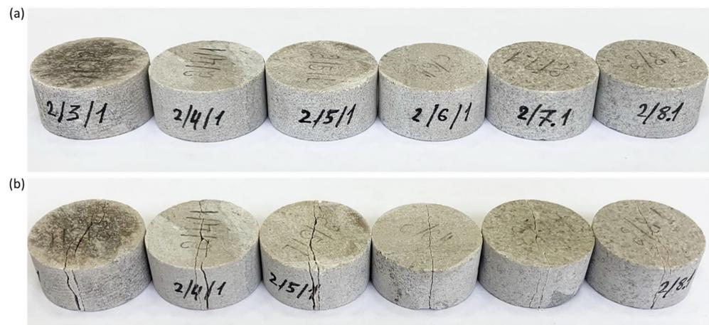
**Figure 10.** Photographs depicting air-dried limestone samples during indirect determination of the tensile strength through the Brazilian test: (a) samples before testing; (b) samples after testing.
