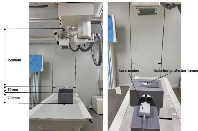
**Figure 2.** X-ray shielding performance evaluation method.
