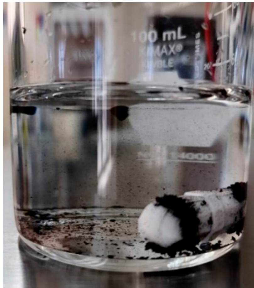
Figure 5. Magnetic properties of biochar (BCM Fe ).
