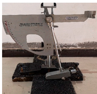
Figure 6. British pendulum test.
