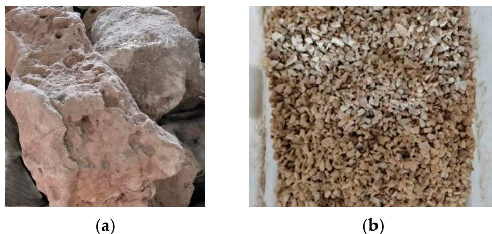
Figure 1. Reef limestone aggregate. (a) Original reef limestone; (b) reef limestone aggregate.
