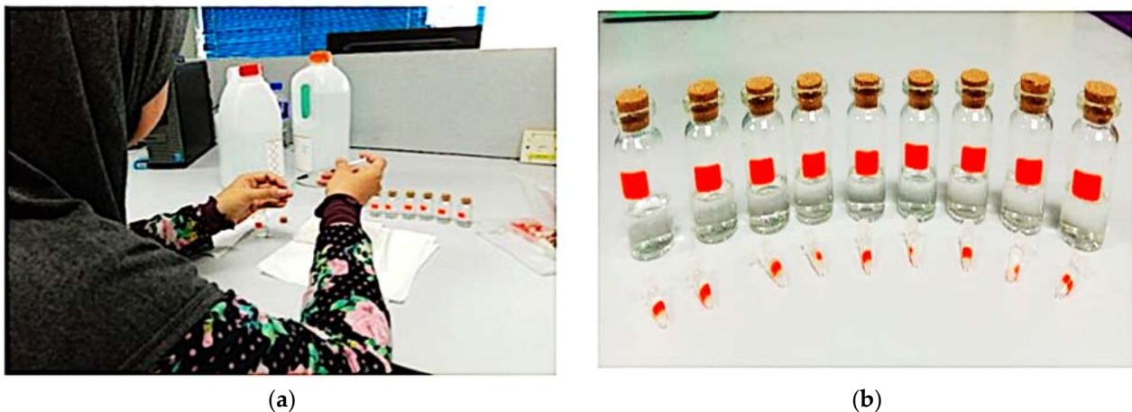
Figure 14. Ethanol–distilled water solutions' preparation: (a) Fill the solution into a PP tube; (b) Ratio of the ethanol–distilled water mixture.
